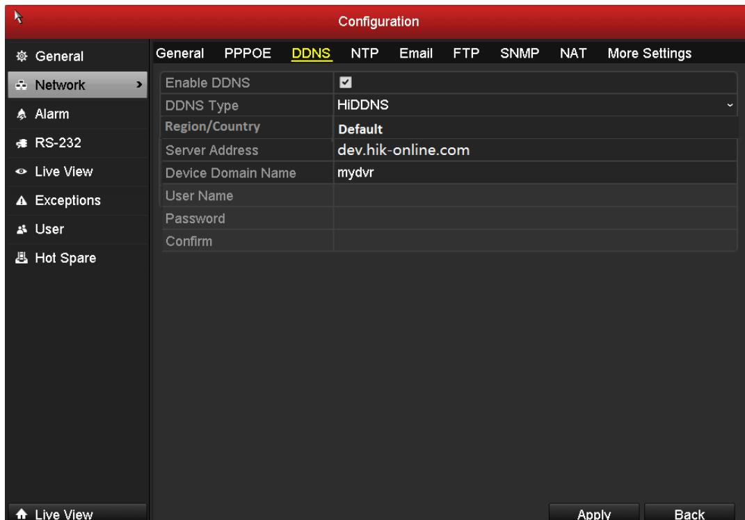
After Apply, if it shows nothing, means successful register. If it shows "Communication to the server failed", please double check the network and DNS settings.
