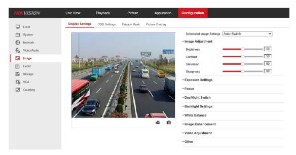
Newly add Auto mode of BLC (Backlight Compensation) Area. When enable HLC (High Light Compression) and auto mode BLC Area at the same time, HLC works, auto mode BLC does not work.
